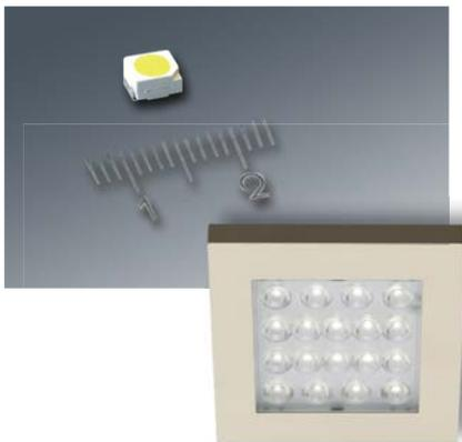
With the SMD „Surface Mounted Device“ style, the component is adhered directly to the printed circuit board. The output ranges differ considerably here. On many LEDs with a small single-power source, series resistors can be accommodated in the luminaire, and connected in parallel to constant-voltage LED transformers (similar to halogen luminaires).
