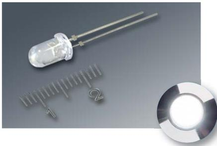
The T-type LED is the original style. Because the sealed casing does not allow heat to dissipate, this style is not suitable for high luminous power applications, but only as a signal/readiness indicator.
