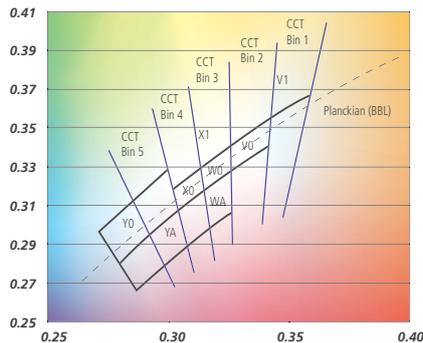
*A binning contains LEDs which are virtually colour-matched.*
