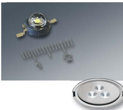
With the SMD type of individual high-output LEDs (here an example of a luminaire with an energy efficiency of approx. 50 lm/W developed in 2003), the luminaires should be connected in series to constant-current LED transformers (unused sockets must be provided with short-circuit plugs).
