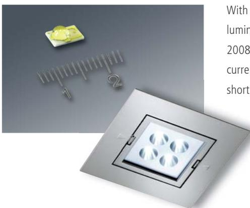
With the new high power SMD-style LEDs (here an example of a luminaire with an energy efficiency of 80 - 100 lm/W developed in 2008) the luminaires should also be connected in series to constant-current LED transformers (unused sockets must be provided with short-circuit plugs).
